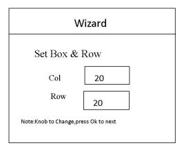
Note: Number of rows/columns in the box refers to the number of horizontal/vertical receiving cards used in the large screen.
