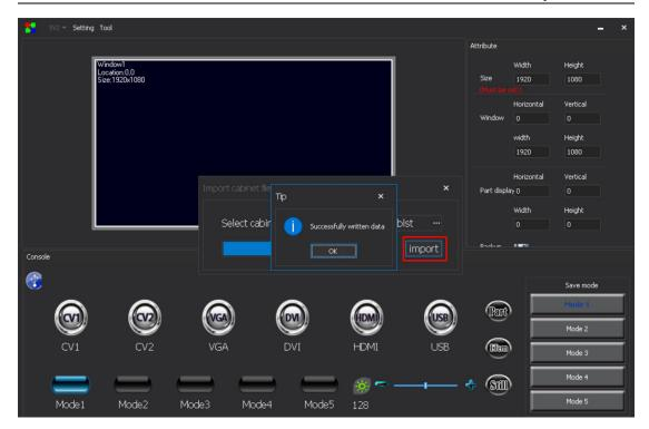
After the software prompts that the data is successfully written, it can be debugged by the video processor. When the processor selects the box file, the imported file file will be displayed on the LCD screen.
